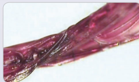
VIS image of nylon microfilaments exposed to freshly drawn bovine blood (5 units heparin/ml) for one hour
